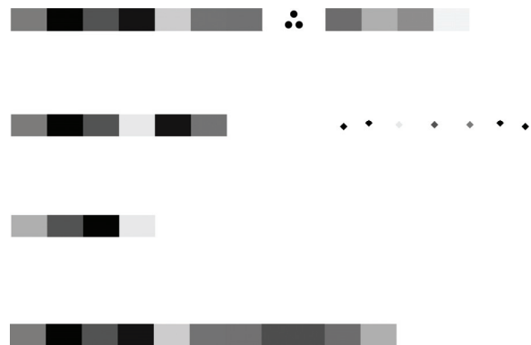
Figure 2 Control strip for density value control for testing printing results on the R2 machine
