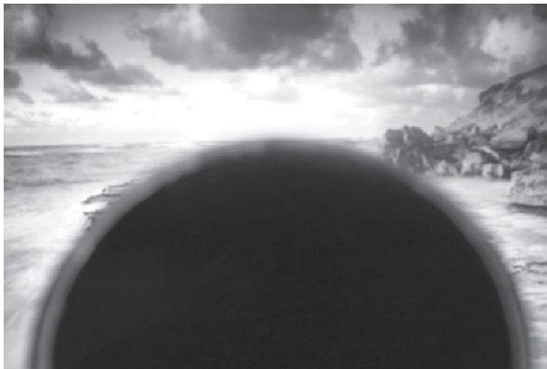
Fig. 1. Light coming from the laptop does not pass through the analyzer
